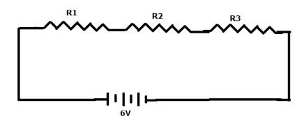
The values of resistors R1, R2, and R3 are respectively 2  $\Omega$ , 4  $\Omega$  and 6  $\Omega$ . They are connected to a 6 volt battery, then calculate (a) the total resistance of the circuit (b) the total current flowing in the circuit (c) current through each resistor.
